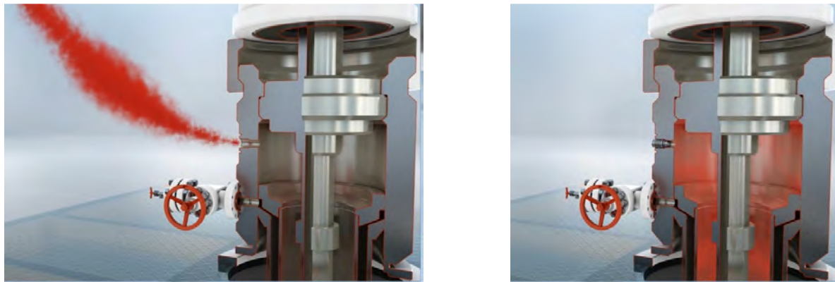
Figure 8 : Damaged annulus outlet showing with and without VR safety valve
